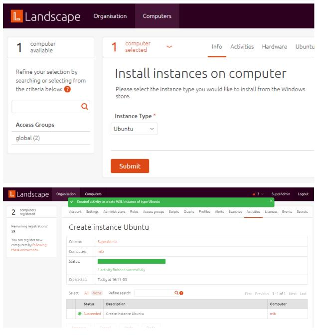
The Landscape server will talk to the Landscape client built into your UP4W. UP4W will then install the Ubuntu application and create an Ubuntu WSL instance automatically. In PowerShell, run ubuntu.exe to log in to the new instance.
